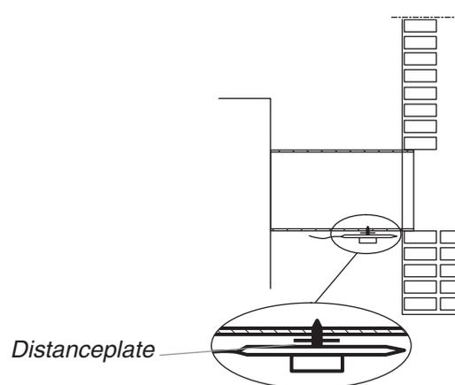
On boilers with low flue-gas temperatures, the probe should be fitted on the side or on the upper part of the flue without distance-plate.
